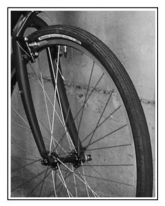
**New for 2017:** We've designed a new light-weight, but still rugged fork for the Phinney Ridge. This drops 3/4 of pound from the front end, and allows for design of the bike in 700c, 650b, or 26" wheel sizes and REALLY wide tires with fenders if desired. The Phinney Ridge has evolved into the most versatile Gravel Bike design as well as one of the lightest on the market.
