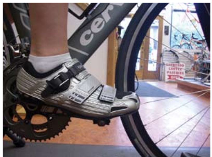
Example of 'toe overlap' on a small bike that uses 700c wheels
