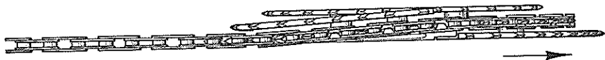
Illustration #10: Top View of Chain Being Switched Up to a Larger Sprocket
