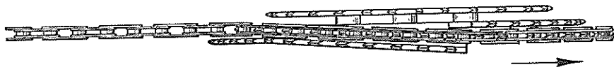
Illustration #9: Top View of Chain Being Switched Down to a Smaller Sprocket
